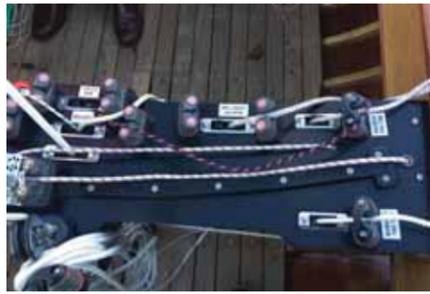
**Control positioning:** Controls will basically be either on a beam under the coachroof or on the mainsheet horse. It is very much a matter of choice what goes where though it will be influenced by the ability to run ropes under the cabin and cockpit floors. However, some are more obvious than others:
