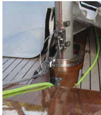
mast to the ram in the coach roof. Most rams have a single line which provides a positive movement in either direction though an alternative is to use powerful shockcord to pull the mast forward.
